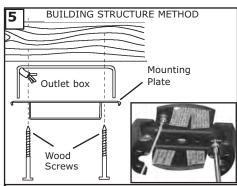
Secure mounting plate directly to a joist from the buliding structure via the two knock out holes on the outlet box. Use only the appropriate wood screws and washers included with your fan. Caution: Wood screws must go through into the building joist.
